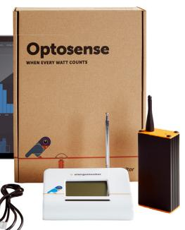
The Energomonitor Optosense set measures the electricity consumption and production of the supply point by reading the optical impulse output on a digital electricity meter.
